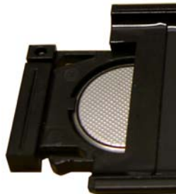
Figure 3: Slide Battery Compartment into Remote
